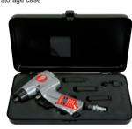
Technical data: Square drive: Max. tightening torque: 40 Nm 1 = 10 Nm Max. loosening torque: 2 = 20 Nm 3 = 30 Nm 4 = 40 Nm 7500 r.p.m. No load current: < 2.69 ms<sup>2</sup> Vibration: Noise performance level: 104 dbA 88 dbA Noise pressure level: Recomended torque: 42 Nm Air consumption: 128 l/min Operating pressure: max. 6,3 (90 psi) Max. screw size: M16 Min. tube diameter 3/8" - 10 mm Connection thread: 1/4"PT
