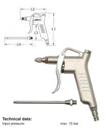
Operating pressure: max. 6,3 bar (90 psi) Max. flow rate: 130 l/min Noise pressure level: 90 dbA Connection thread: 1/4"PT
