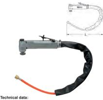
2000/min Oscillating spee 22000 r.p.m. No load current: Vibration: 4.3 m/s<sup>3</sup> Noise performance level: 79.8 dbA Noise pressure level: 69.9 dbA Air consumption: 300 l/min Operating pressure: 6,3 bar (90 psi) Min. tube diameter: 3/8" - 10 mm Connection thread: 1/4"PT
