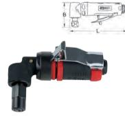
Technical data: 6 mm Capacity: 190 Watt No load current: 19000 r.p.m. Vibration: < 1.5 ms<sup>2</sup> Noise performance level: 95 dhA Noise pressure level: 82 dbA Air consumption: 240.66 l/min Min, tube diameter 1/4" - 4.8 mm Operating pressure: max. 5,5 bar (80 psi) Connection thread: 1/4
